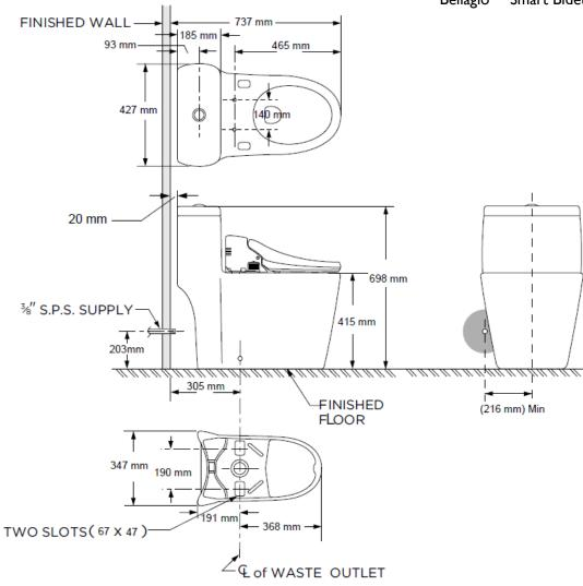
THIS FIXTURE QUALIFIES ACCORDING TO ASME TEST PROCEDURES AS A LOW CONSUMPTION WATER CLOSET WITH AN AVERAGE CONSUMPTION OF 1.6 gpf (6.0 Lpf) OR LESS.
