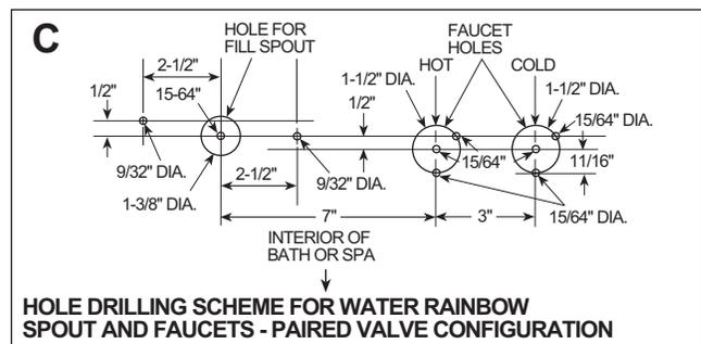
Using a scribe tool or awl, mark the center points for all holes, then remove the template.
