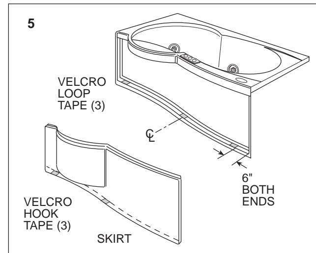
6. Lift the top of the skirt up under the rim of the bath, center the skirt in the opening, then swing bottom of skirt onto rail. The Velcro® on the skirt and the rail should mesh. See illustration 6.
