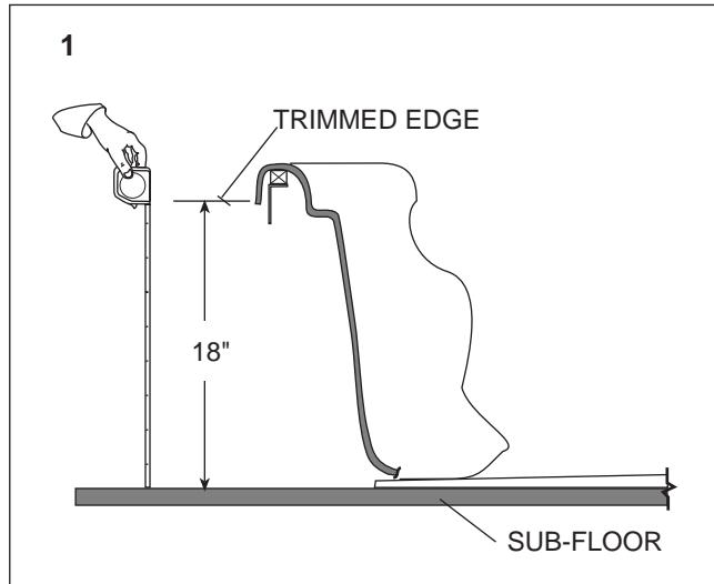
1. The bath should be set and levelled according to the installation instructions. Electricity should be connected and bath system tested to be sure it is working properly without leaks before installing the frame and skirt. The installation dimension from the sub-floor to the trimmed edge of the bath should be 18 inches. See Illustration 1.
