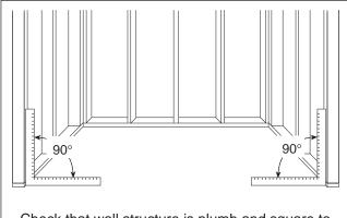
Check that wall structure is plumb and square to the floor. Shim the framing if necessary before finishing to ensure a square opening.
