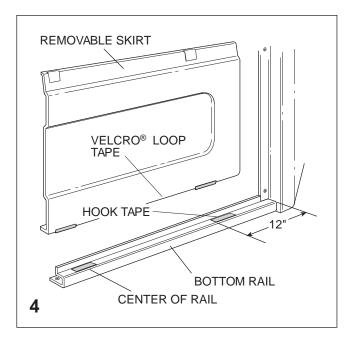
Lift the top of the skirt up under the rim of the bath, center the skirt in the opening, then swing bottom of skirt toward the rail and lower skirt onto rail. The Velcro® on the skirt and the bottom rail should mesh.
