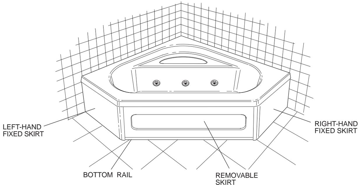
The optional skirt is designed to allow the minimum service access necessary to the motor/pump and plumbing of the bath and consists of three pieces; left-hand fixed, right-hand fixed, and removable front panel, along with the necessary bottom rail and hardware for installation. (See the Illustration above.)
