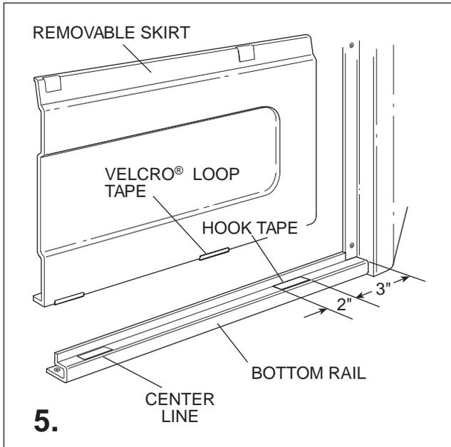
Clean an area about 2" long in the center, and 3" from each end of the rail and the bottom of the skirt with isopropyl alcohol. (See illustration 5). Attach strips of Velcro®, as before, hook tape to rail, loop tape to skirt, ensuring that they will mesh when the skirt is installed.
