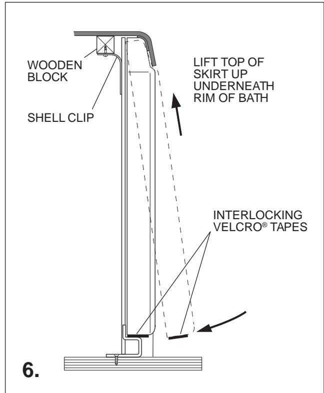
Lift the top of the skirt up under the rim of the bath, engaging the clip. Swing the bottom of the skirt in towards the rail and lower the skirt onto it. The Velcro® tapes will mesh, holding the skirt in place. Proceed with the installation of the wall and finished flooring materials.
