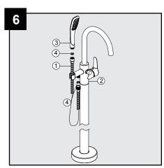
Connect one end of the shower hose (1) to the mixer (2) and the other end to the hand shower (3). Ensure the washer (4) is in each end for seal.
