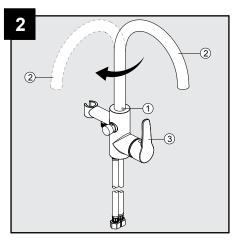
Loosen the set screw (1) pre-assembled to the spout (2), rotate the spout (2) about 90° to align handle (3), then tighten the screw.
