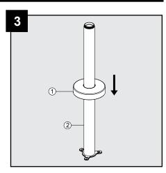
Place the escutcheon (1) over the standpipe (2) and then push it to the base.
