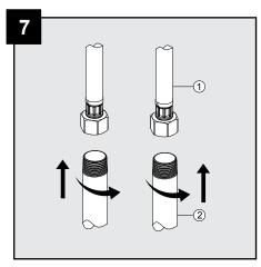
Connect the flexible supply lines (1) to the water supplies (2).
