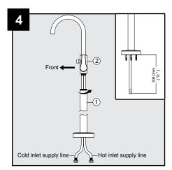
Screw the standpipe (1) onto the mixer (2) by hand. Turn in a clockwise direction until it is tight. Note1: Do not to reverse the cold and hot supply lines. Note2: After installing the standpipe (1),the inlet supply lines exposed 12 in.,we need to pay attention to set aside enough space to connect the water inlet supply lines to prevent the water inlet supply lines from twisting.
