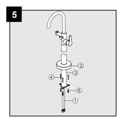
Place the assembly with the flexible supply lines (1) through the prepared hole and then holding the escutcheon (2), secure the standpipe (3). Note: If mounting into wooden floor, secure the standpipe (3) using screws (4) only (wall plugs are not needed). If mounting into solid floor, mark the position of holes first and then secure the standpipe (3) using anchors (5) and screws (4). Where requried ensure correct anchors for your floor type are used.
